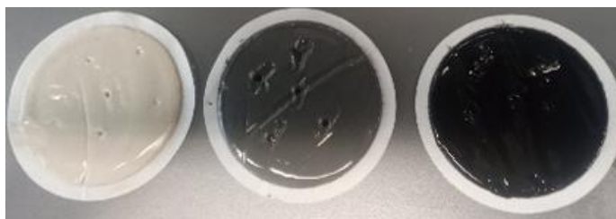
Figure 4: Close-up of Fresh Filter Cakes Post-Filtration: (a) Base Fluid, (b) GO 0.1 wt.%, (c) GO 0.45 wt.%.
